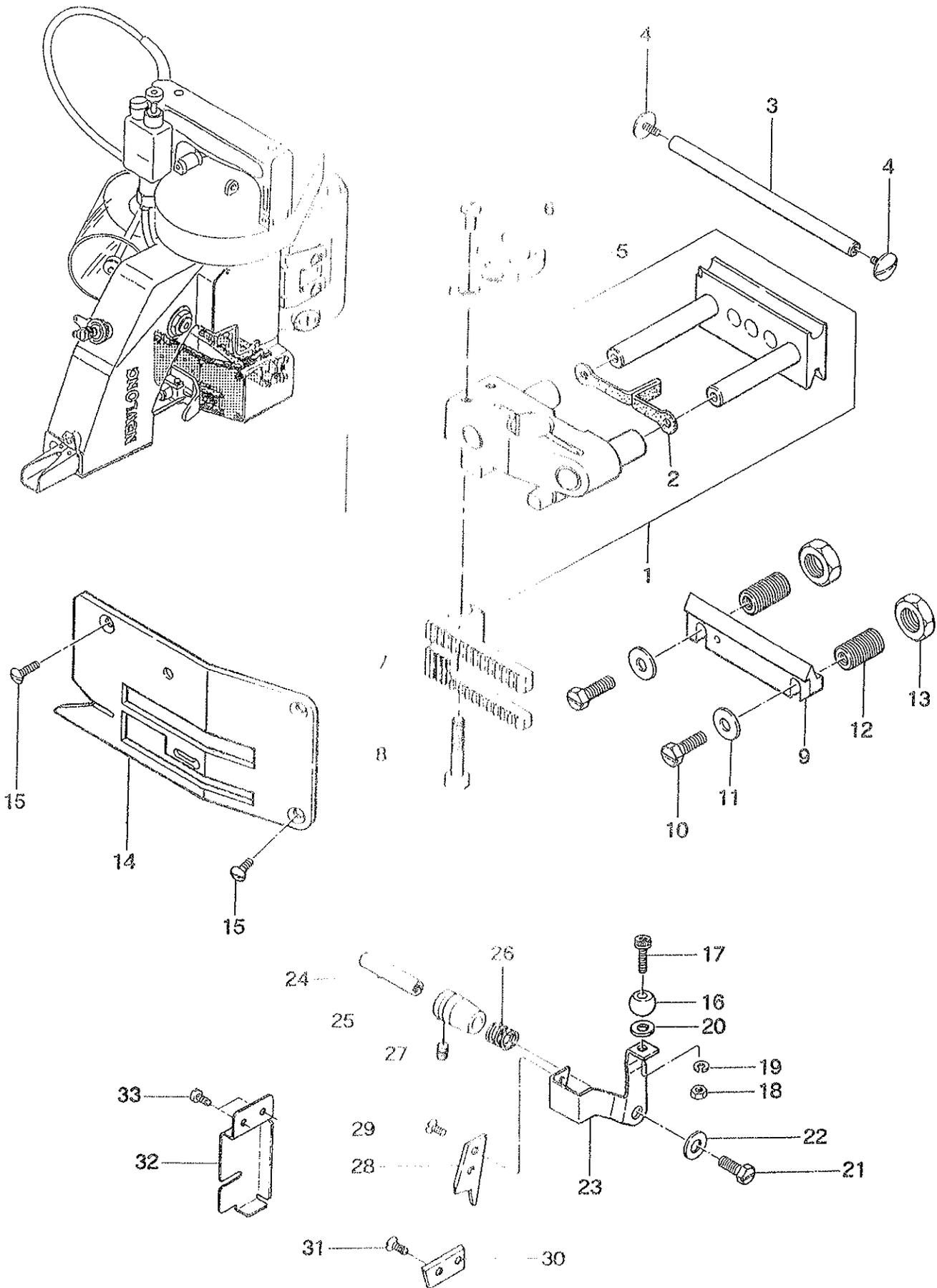
(5) FEED DRIVING AND THREAD CUTTER PARTS
